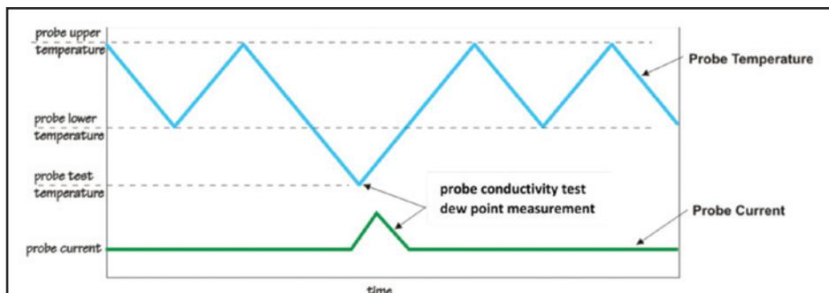
**Fig. 6: Breen-SA Probe normal cycle and check cycle.**
