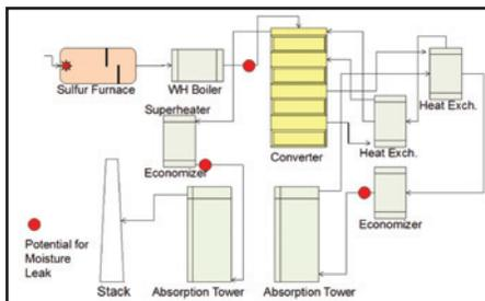
Fig. 1: Typical moisture ingress points in sulfuric acid manufacturing.
