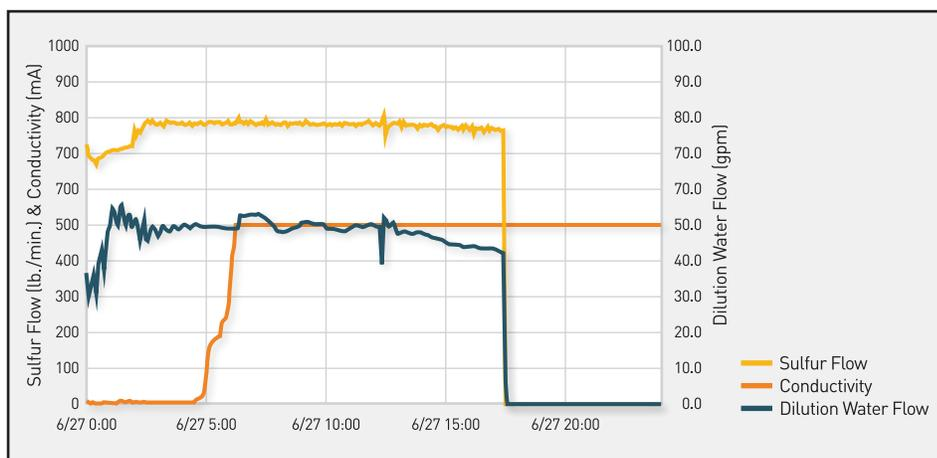
**Fig. 8: Leak detection from Breen-SA Probe vs. dilution water flow.**
