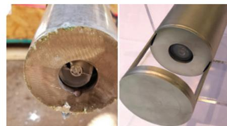
**Fig. 9: During installation, SA Probe sensor, left, damaged from obstruction in port. At right, sensor protective shield.**
