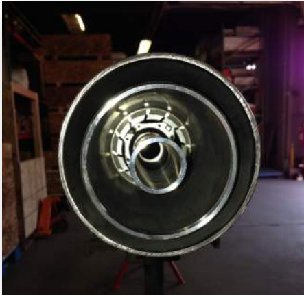
Above – End view of an 80 mmBTU total throughput Dual Orifice Igniter
