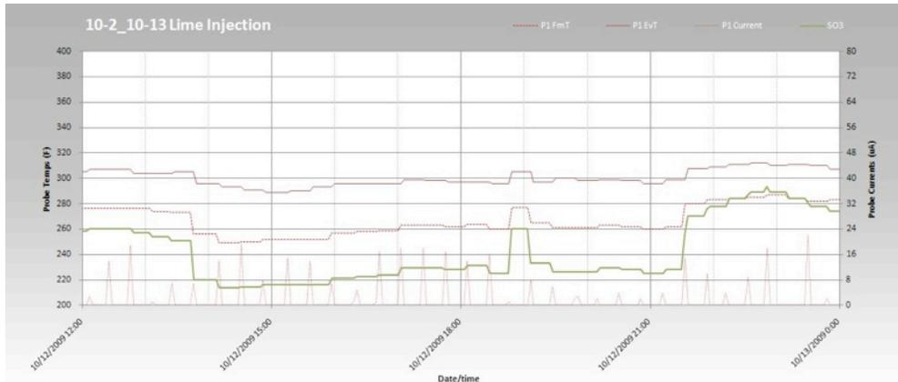
**Figure 3 - Results of Pre-SCR Hydrated Lime Injection**
