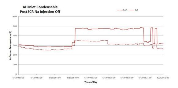
The third graph below shows the effect of startup of the post SCR Na injection point with the post SCR flue gas initially in an ammonium bisulfate state.
