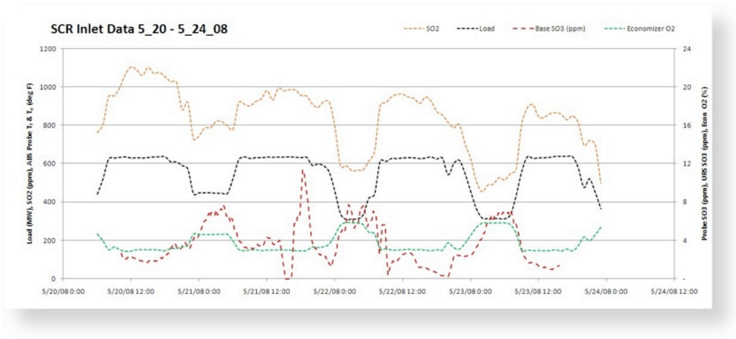
Figure 4 - Economizer Outlet SO3 vs. Load & O2
